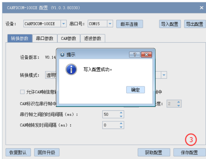
Figure 5.5 Saving the configuration
