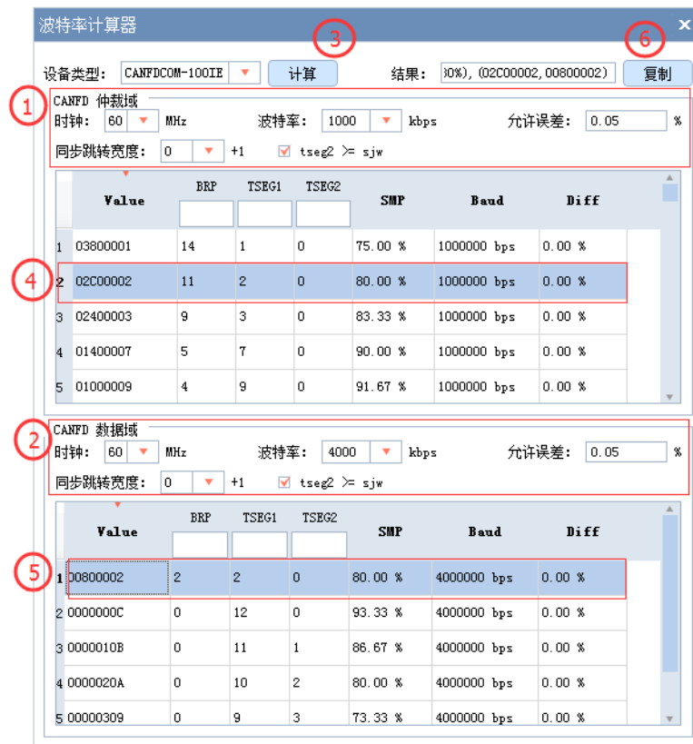
Figure 3.5 Steps for using the baud rate calculator
