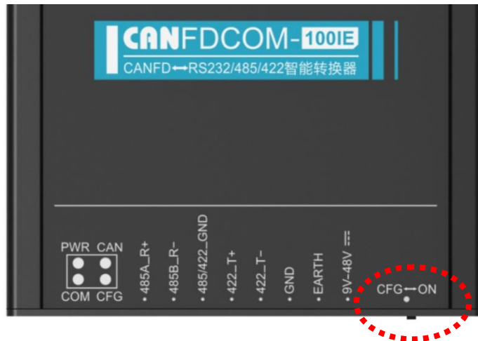
Figure 5.1 Entering the configuration mode
