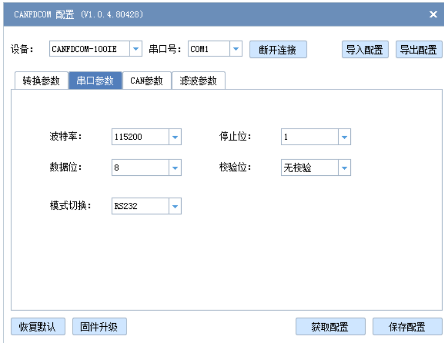
Figure 3.3 Serial port parameter settings
