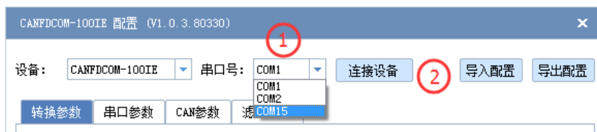
Figure 5.2 Connecting a device
