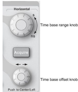
Figure 3-3: Horizontal control area
